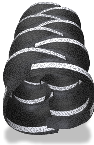
Fig. 4.8: Simulation of a pattern of parallel ribbons rolling into a cylinder.
