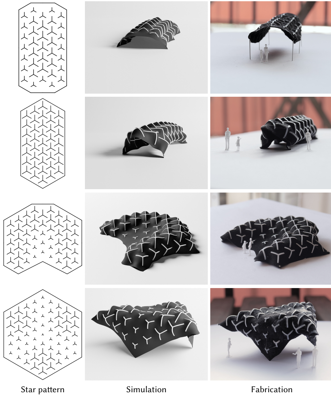
Fig. 3.9: Various architectural models created using our system, from top to bottom: a U-shape, a tunnel and a doubly-curved roof. For each result we provide the star layout to be printed (left), the simulated surface (middle), and the printed result (right).
