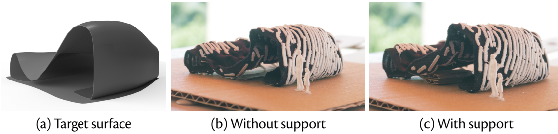
Fig. 5.13: Limitation. Without additional support, this architectural model sags under its own weight (b). Adding a cardboard support underneath the structure brings it closer to the target surface (c).
