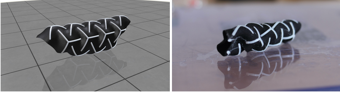
Fig. 3.2: Our simulation tool (left) correctly predicts that a uniform star pattern, with free boundary, rolls up into a cylinder at static equilibrium (right). This complex behavior is due to the extrinsic curvature induced by the bilayer structure of the ribbon-and-fabric assembly, and the coupling of the bending of neighboring stars causing global symmetry-breaking in the pattern.
