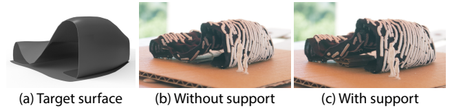
Figure 12: Limitation. Without additional support, this architectural model sags under its own weight (b). Adding a cardboard support underneath the structure brings it closer to the target surface (c).
